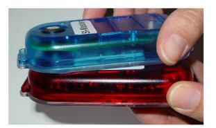
**8.** Place the station on the coupling stick and the SI-Master. After some seconds there is a 'beep'. The time of the station is now adjusted.
